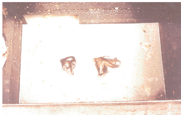
machine fluid sump with food debris (teabags)
